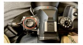
Then there are the two buttons on the cap of the on off lever on the left side of the top of the camera. The front one gives you access to your drive mode settings. Want to switch to SH1 or SH2 for a burst of intense action or a fast flying bird. Press the button and rotate the rear wheel. Do the same if you want to try one of the ProCapture modes.
